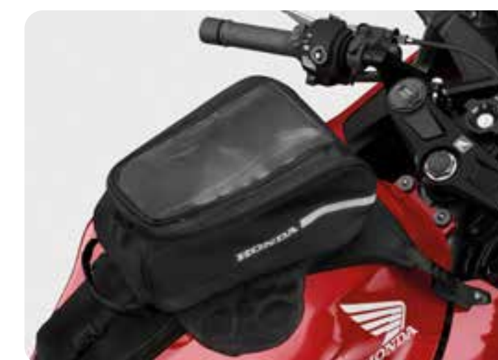
TANK BAG 08L71-MKJ-D00 Practical 3L tank bag featuring a clear pocket on top for a convenient smartphone storage. Easy to fit, this tank bag doesn't interfere with the handling of the motorcycle. Rain cover is included. Dimensions in mm (W x L x H): 178 x 285 x 130. Tank Bag Attachment sold separately.
